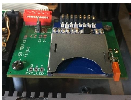
A board with a single SD slot installed in place of a Microdrive
