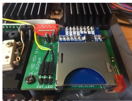
A board with two SD slots installed in place of a Microdrive
